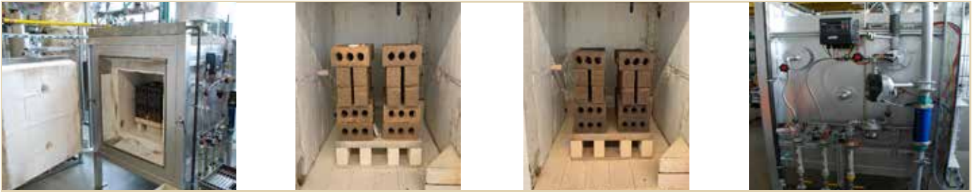
Laboratory kiln for firing trials with varying atmospheres
