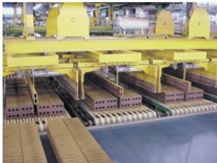
The transfer gripper picks up eight double rows and transfers them onto four marshalling conveyors, where they are grouped and held in position for the setting plant.
