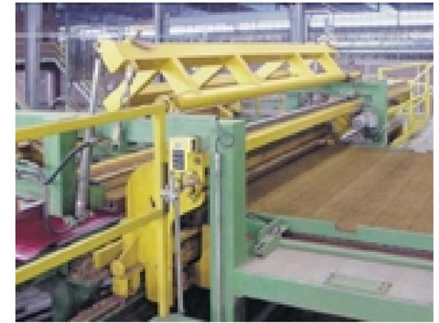
The continuously formed clay column is cut off initially at a length of 18 feet and measures 8" x 4" in cross-section. The column is chamfered and provided with a textured surface. The clay slugs are doubled up adjacent to each other and cut exactly to size in a push-thru multi-wire cutter.
