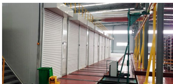
附自动摆渡车的室式干燥机 Chamber dryer with automatic transfer car
