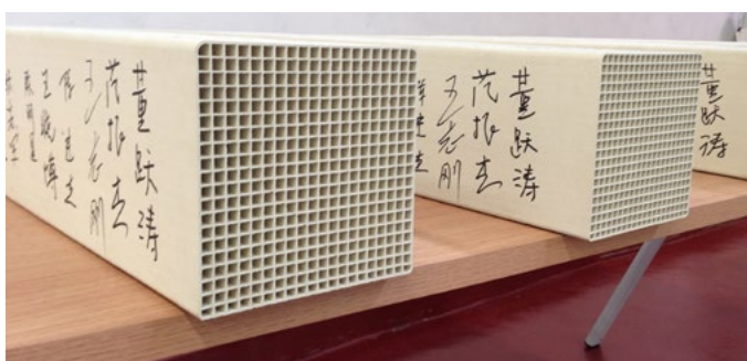
最先从新厂生产出来的催化剂 First catalysts out of the new plant
