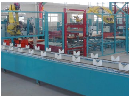
催化剂输送线 Catalyst conveyor
