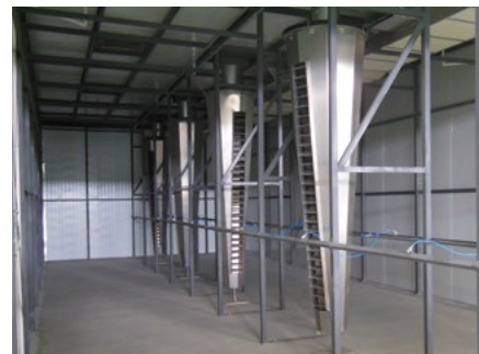
室式干燥机内部的旋转风机 View inside a chamber dryer with rotary fans
