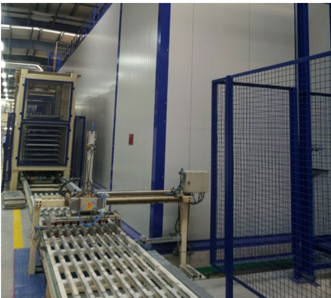
有托盘回转输送线的干燥机入口 Dryer entrance with pallet return conveyor
